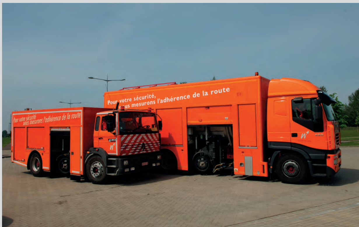
Le SCRIM (Sideway-force Coefficient Routine Investigation Machine). © SPW-Direction de l'Édition
